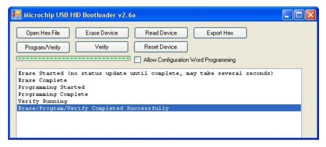
Now remove the link between pin1 and 0v ground and press "Reset Device". This will reset the module and run your application.
