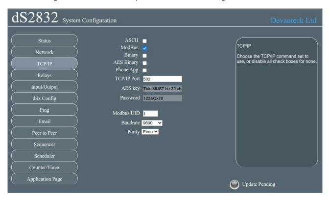
These allow you to select the UID, normally you will leave this at the default of 1. The dS2832 will respond to commands on this UID. If you send any other UID it will be treated as the address of a Modbus module connected to the RS485 port. Commands to other UID's will be converted to Modbus RTU format and sent out on the RS485 port. Any responses will be converted back to Modbus/TCP format and returned to you.
