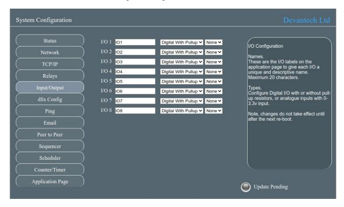
As with relay names these may be up to 20 characters long, but do check it looks ok on a mobile device or whatever you are using to control the module.
