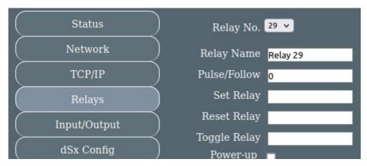
If you want, you can give the relay a more descriptive name. To use input 161 as an analogue input we use A161. If we wanted a digital input it would be D161. Enter the following into the Pulse/Follow box:
