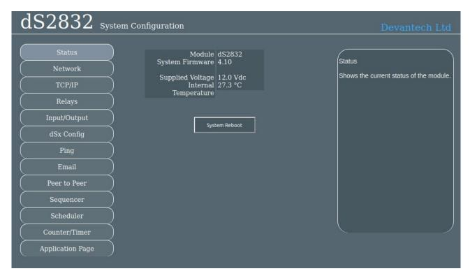
This status page shows you the system and application firmware revisions as well as the supplied voltage to the board and its internal temperature.
