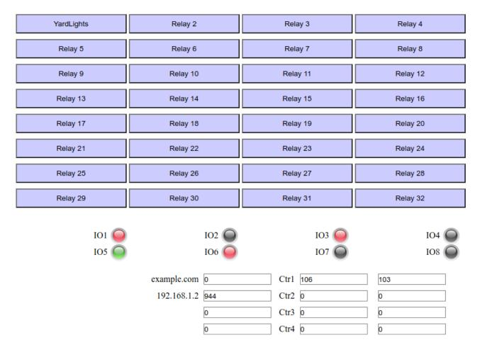
The I/O indicators show grey when the I/O is inactive. When an active input is applied they show green. Red indicates an active output from the module.
