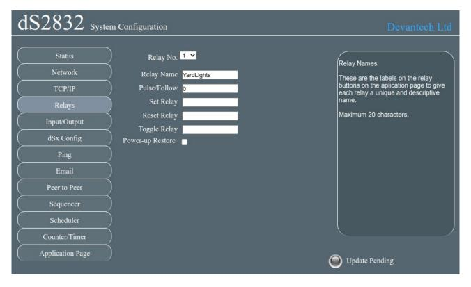
Use the Relay No. box to select the relay to configure. There are 32 relays available. Unlike other dS modules the dS2832 does not have virtual relays. All relays 1-32 are the physical relays, however I/O lines may still be be linked to relays to provide additional physical outputs, see next section for details.
