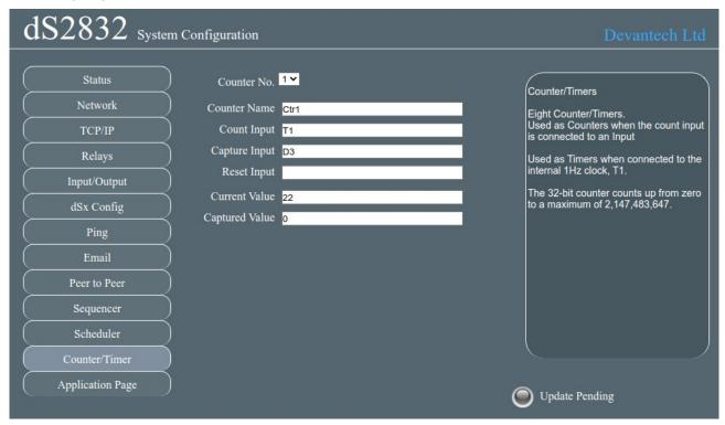
There are a total of eight counter/timers available, selected with the Counter No. box. Each counter can count at a maximum speed of 10Hz (10 counts per second).
