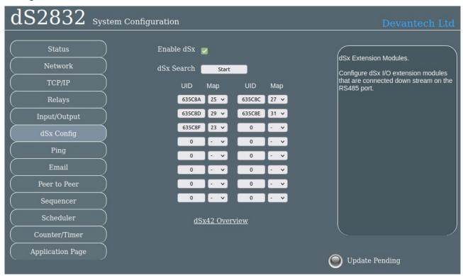
dSx mode is enable by checking the Enable dSx box. This will configure serial port 3, the RS485 port, to 250k baud as used by the dSx modules. If un-checked the port will be configured to the Modbus settings on the TCP/IP page. Reset the board after checking or un-checking this box.
