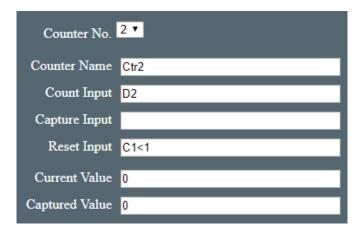
The count input is set to D2 to count the pulses. The reset input is controlled be counter 1. When it gets reset to zero each hour, so does counter 2. As the capture input is blank the reset event also captures the count value. This may be read any time in the next hour.
