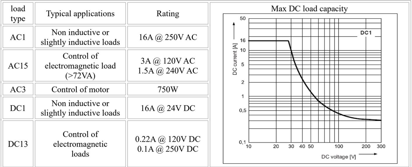
A full datasheet for the relays used on the ETH1610 is here: [HF115FD datasheet](#)
