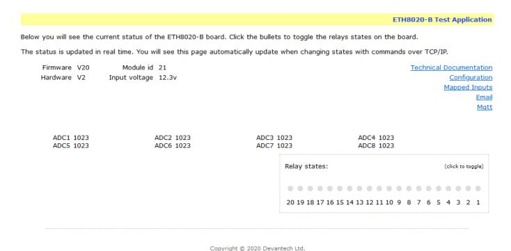
This web page will allow you to switch the relays on and off by clicking the relay buttons (the red/gray circles). It also contains a links to this technical documentation page, the network configuration, mapped inputs, email and mqtt.
