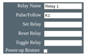
Placing K1 in a relays Pulse/Follow box will make the relay follow the K1 output, in this case pulsing the relay on and off every two seconds.
