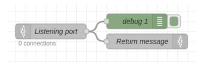
A tcp in node is connected to a tcp out node and a debug node. The tcp in node is set to listen on the selected port. The tcp out node is set to "Reply to TCP". The debug node allows you to see the message being sent. We used this setup to generate the message screenshot above.
