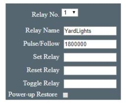
The above example will turn off the yard lights after 30 minutes. 1800000 mS is 1800 seconds. 1800 seconds is 30 minutes.
