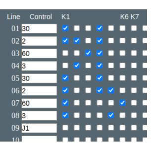
Here we hold both lights at Red for 30 seconds to give traffic time to traverse the controlled area. Then Red + Amber for two seconds followed by Green for 60 seconds. We then stop the traffic with Amber for 3 seconds followed by Red. Again we hold both lights at Red for 30 seconds before letting the other queue through at line 6.
