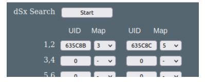
Next change the mapping as required to 29 for the first module and 31 for the other, using the drop-down selection boxes.
