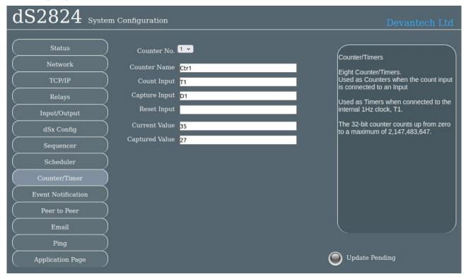
There are a total of eight counter/timers available, selected with the Counter No. box. Each counter can count at a maximum speed of 10Hz (10 counts per second).
