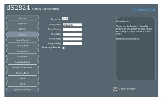
Use the Relay No. box to select the relay to configure. There are 32 relays available. Relays 1-24 are the physical relays on the module. Relays 25-32 are virtual relays, they have no physical presence but otherwise behave the same as the real ones. I/O lines may be linked to virtual relays to provide additional physical outputs, see next section for details.
