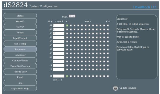
The sequencer runs a continuous loop of up to 120 steps. At each step you can specify a time delay and the outputs. The K1 – K12 outputs are updated and the start of the delay time. The example above shows the simplest sequence possible. At line 01 it delays 1 second and turns on the K1 output. Line 02 delays 1 second and turns off the K1 output. Line 03 jumps back to line 1 and the cycle repeats forever.
